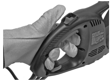
Figure 3-8: Releasing trigger switch to stop trimmer
